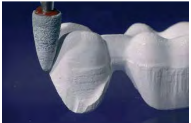
Use suitable grinding tools to finish/adjust the non-sintered framework.
