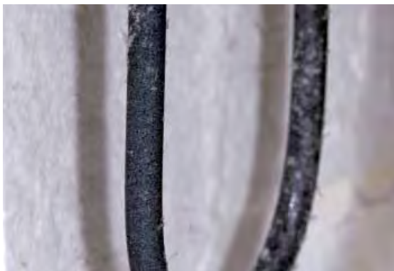
Contaminated, severely corroded heating element
