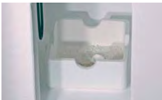
Align the firing sagger with the positioning pins.
