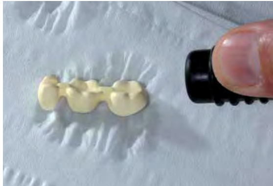
Blow dry the framework with oil-free air.
