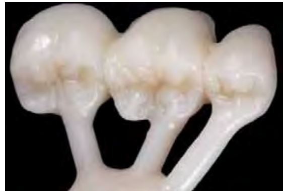
Rough divestment is carried out with glass polishing beads at 4 bar (60 psi) pressure until the objects are visible. For fine divestment, apply 2 bar (30 psi) pressure.
