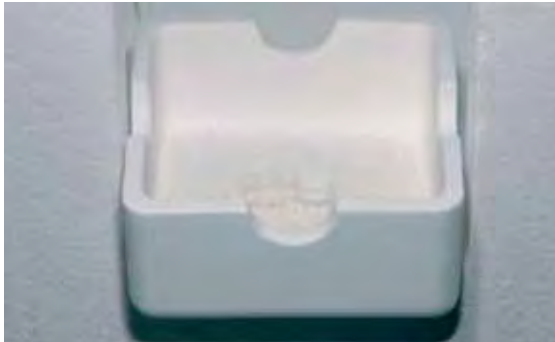
After completion of the sintering process, allow the firing sagger to cool to room temperature and remove it from the Sintramat.
