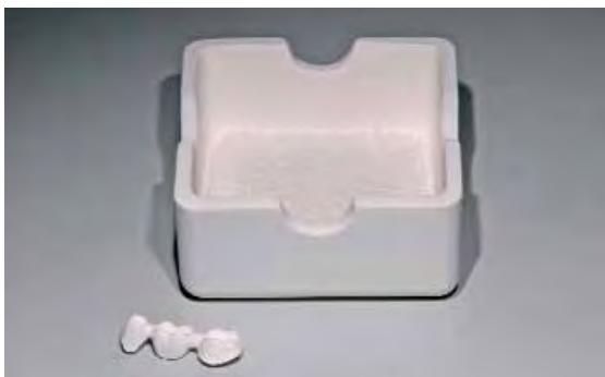
Firing sagger filled with 100 g ZrO 2 beads.
