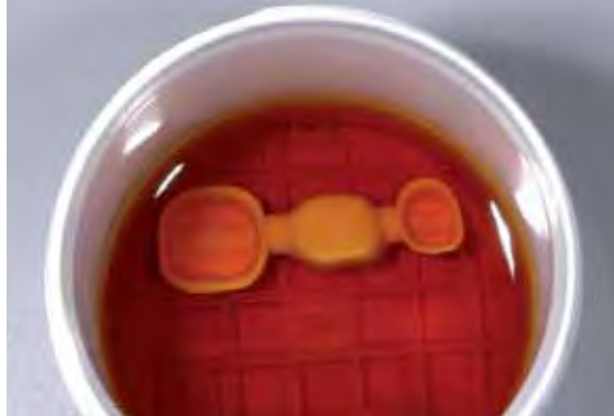
Dip the framework into the Colouring Liquid for 2 minutes to ensure a penetration of a wall thickness of 0.7 mm.
