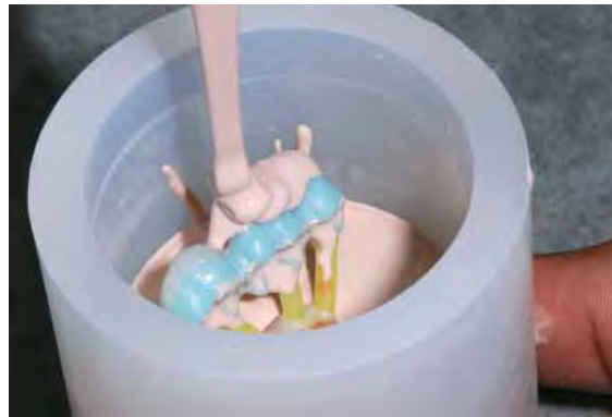
Provide sprues on the IPS e.max ring base always in the direction of flow of the ceramic and at the thickest spot.
