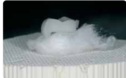
Place the objects on the honey-comb firing tray and start the firing program
