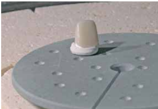
After the crystallization program, remove the firing tray from the furnace and allow the IPS e.max CAD restoration to cool to room temperature.
