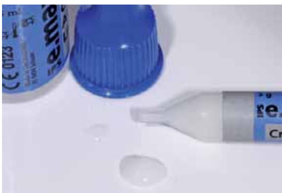
Extrude IPS e.max Crystall./Glaze paste from the syringe and mix thoroughly. If required, slightly thin with the IPS e.max CAD Crystall./Glaze Liquid.
