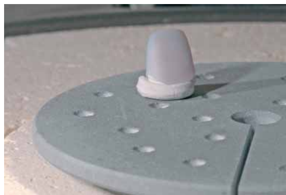
Place the firing tray in the furnace and start the crystallization program.
