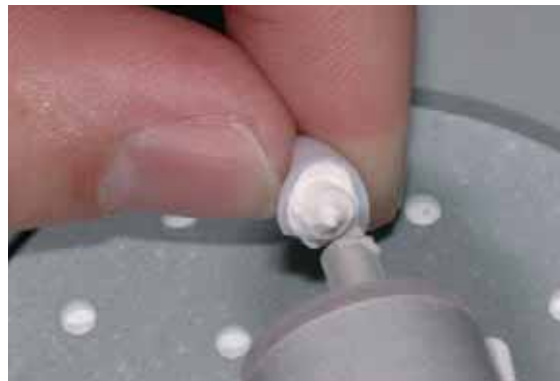
Fill the cavity completely with IPS Object Fix Putty or Flow and attach a base.
