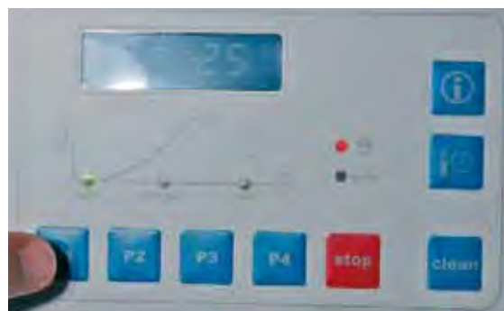
Press P1. The sintering program starts automatically and the furnace door is locked.
