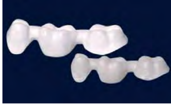
Comparison of a non-sintered and sintered IPS e.max ZirCAD framework.
