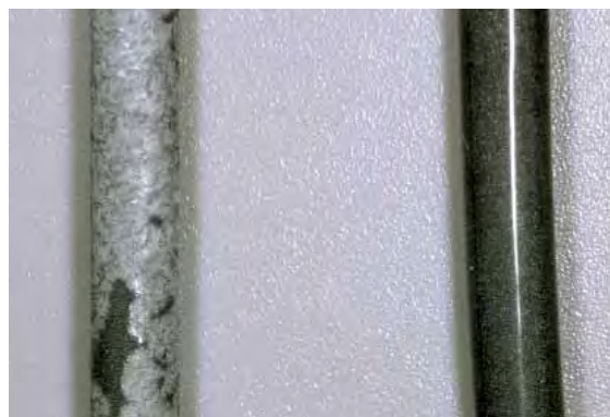
Corroded heating element (left). Repeat the cleaning program several times until the surface of the heating element is free from contamination and appears glassy (right).
