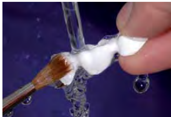
Thoroughly rinse milling dust from the framework under running water. Use a brush, if required.
