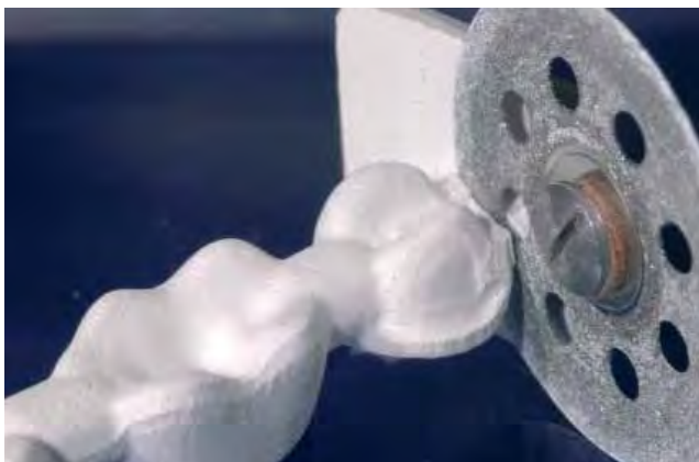
Carefully separate the milled framework from its holder using a separating disk.
