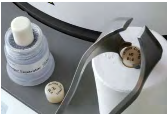
After the preheating cycle, place the cold ingot into the hot investment ring and conduct the press procedure.
