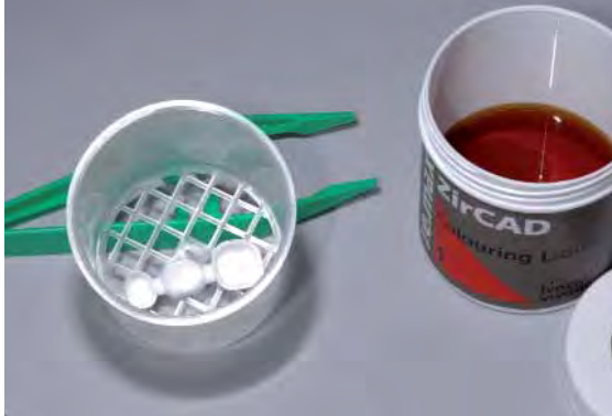
Fill the working cup up to approximately 2 cm with Colouring Liquid and place the dry IPS e.max ZirCAD framework with the occlusal surface facing down in the sieve insert.
