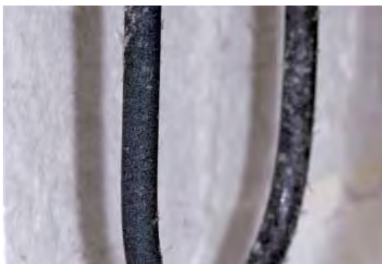
Contaminated, severely corroded heating element
