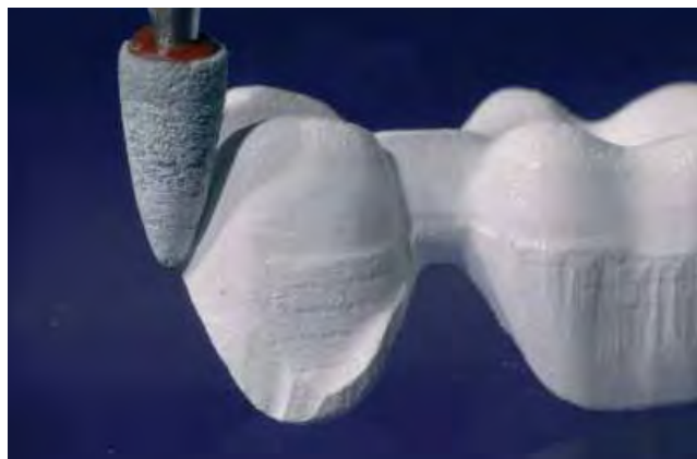
Use suitable grinding tools to finish/adjust the non-sintered framework.
